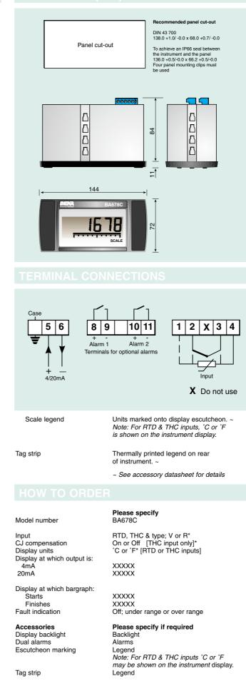
\* If calibration information is not supplied, instrument will be conditioned for 3 wire Pt100 RTD input with a 4 to 20mA output corresponding to a display of 0.0 to 100.0°C.
